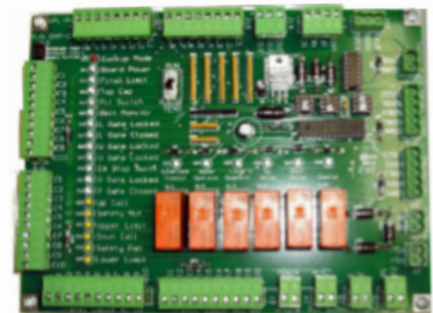
LED Diagnostic Board (located under main tower cap)
